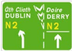
Lane destination sign
