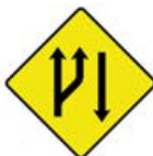
Start of a climbing lane
