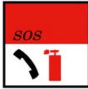
Fire Extinguisher and Telephone
