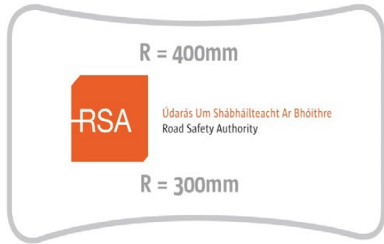
Figure 2: Tool for checking the radius of curvature of the wide angle (Class IV) mirror. (Dimensions shown are in millimetres)
